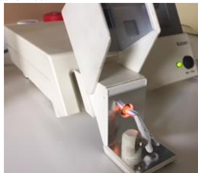
Fig 5: Light box for additional curing.
