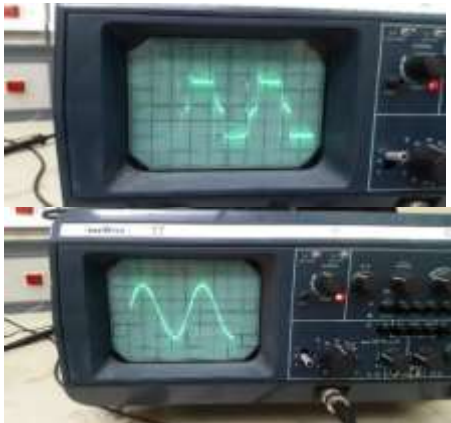
Fig. (12). Effect of the inductive load on the output wave
