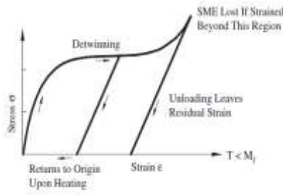
(b) Figure (4): Stress-strain curves for SMAs: (a) super-elasticity effect; (b) shape memory effect. [23]
