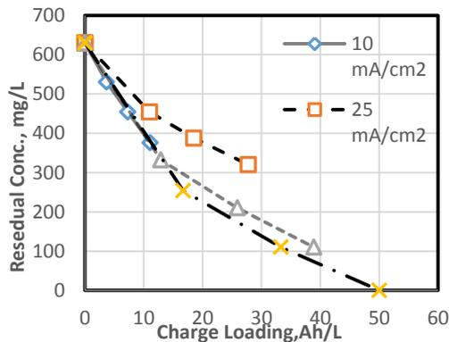
Fig. 4. Effect of current density on the residual concentrations of nitrate (Co= 630 mg/L)
