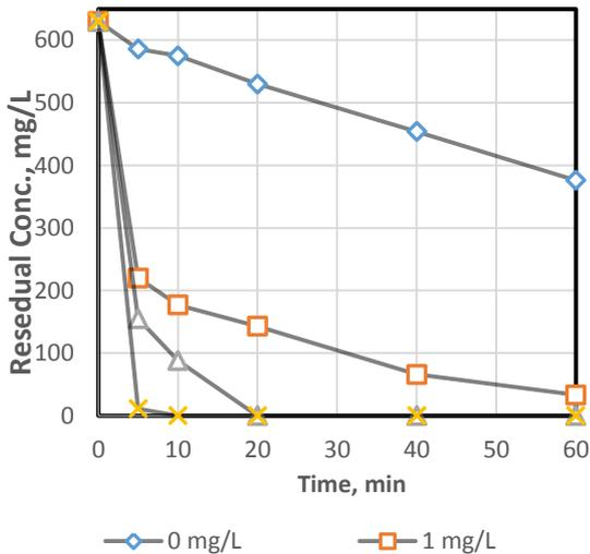
**Fig. 8.** Effect of supporting electrolyte (different concentrations of NaCl) on residual concentrations of nitrate ( $C_0 = 630$  mg/L,  $i = 10$  mA/cm<sup>2</sup>)
