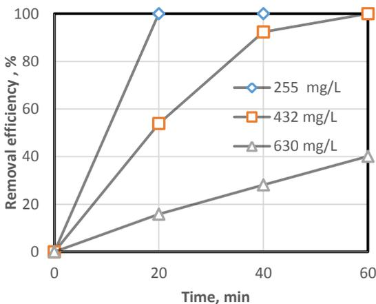
Fig. 6. Effect of initial concentrations of nitrate on the removal efficiency (i = 10 mA/cm<sup>2</sup>)
