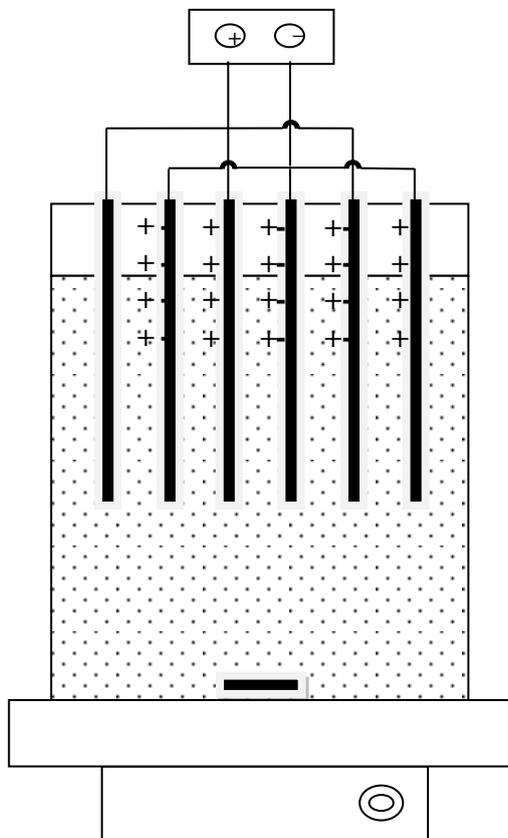
Fig. 1. Bench-scale EC reactor with monopolar electrodes in serial connection.
