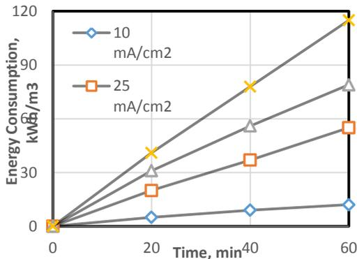
Fig. 5. Total energy consumption values as a function of current density (Co= 630 mg/L).
