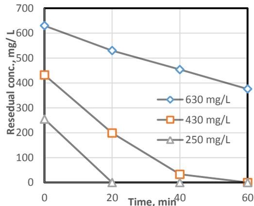
Fig. 7. Effect of initial concentrations of nitrate on the residual concentrations (i = 10 mA/cm<sup>2</sup>)
