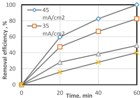
Fig. 3. Effect of current density on the removal efficiency of nitrate (Co= 630 mg/L)
