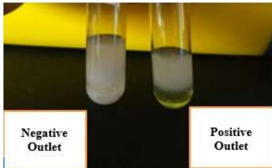
Figure 4. Results of using silver nitrate with 10 kV resulting samples.
