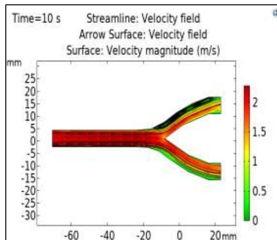
Figure 6. Particles trajectories of COMSOL model without applying electric field.
