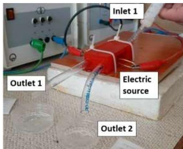
**Figure 2. Separation device with the saline solution pumping and applied external electric field.**
