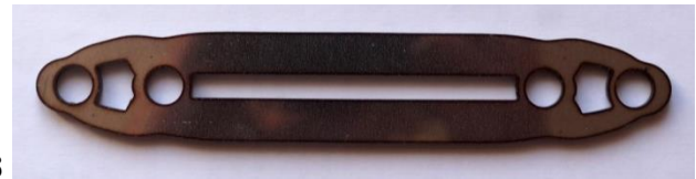
353 354 Figure 3 – Laser-cut prototype of the plate
