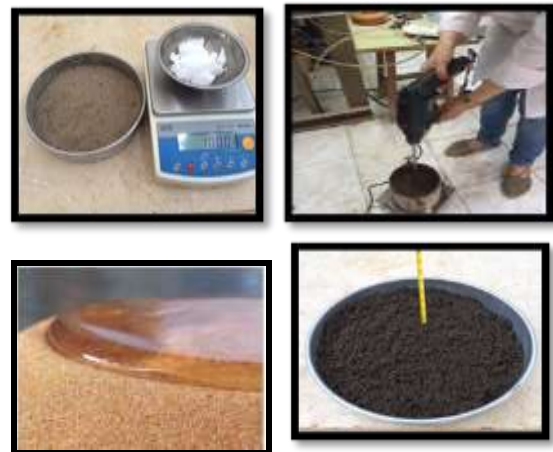
Figure 6: Method of forming wax-coated sand
