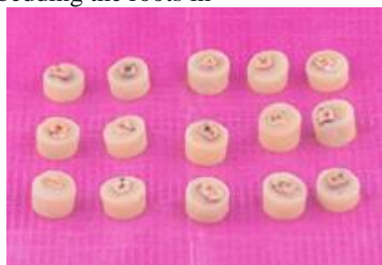
Figure (2): Representative samples fixed in cold-cure acrylic resin molds for standardized testing.
