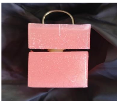
Figure (2): Tooth embedded in acrylic resin molds.
