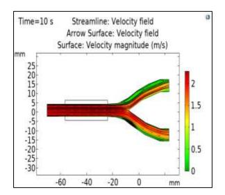
Figure 7. Figure 6. Particles trajectories of COMSOL model after applying electric field in the black rectangle.
