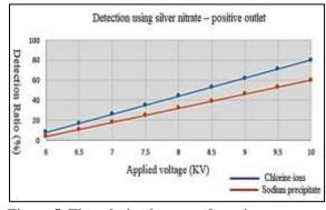
Figure 5. The relation between detection outcomes in positive outlet and applied electric voltage.
